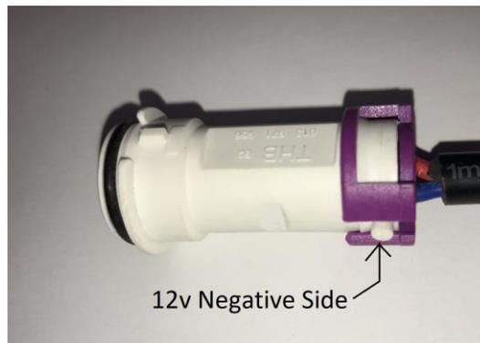
**Note:** During charge only, provides up to 2 amps at 12v DC
