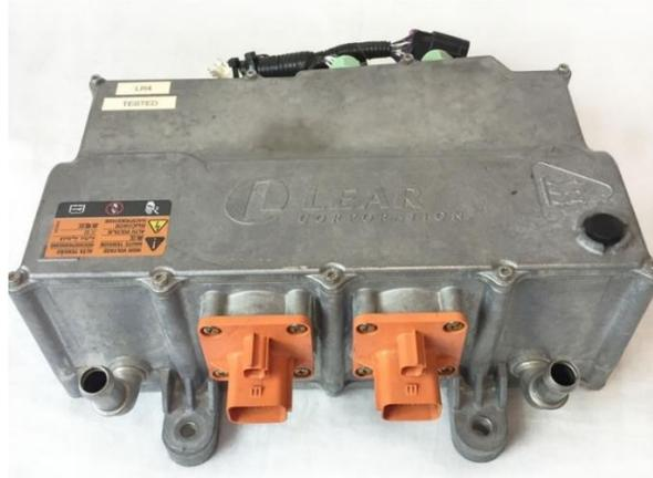
The EVCC CAN wires are included in the kit along with a 120 ohm resistor if tests show it is needed for CAN functionality. Note that the Lear charger has a CAN data rate of 500kbps. The EVCC can be configured with this setting. If using a CAN enabled BMS, it must be configured for a 500kbps data rate.
