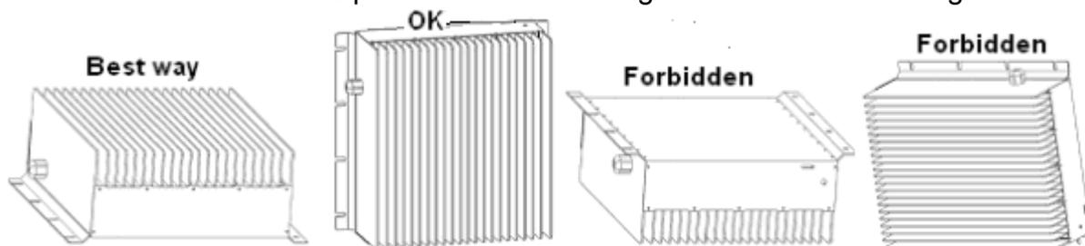
3. Ensure all heat-dissipating parts are not obstructed to avoid overheating. Do not
