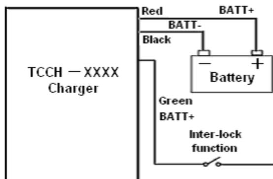
Connect to coil of main contactor, DC/DC converter or controller enable wires. Normally battery voltage +, but OV while charging.
