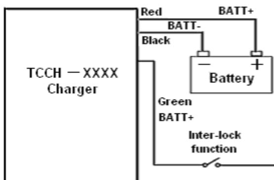
Connect to coil of main contactor, DC/DC converter or controller enable wires.
