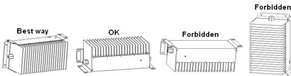
3. Ensure all heat-dissipating parts are not obstructed to avoid overheating. Do not put the battery charger near any heat sources. Make sure that free space around the charger is enough to provide adequate ventilation & easy cable socket access.
