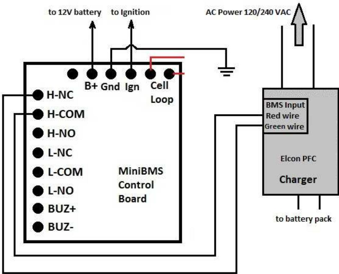
This diagram is for new style Elcon PFC charger with 7 pin round connector, which simply requires closure of Red/Green control wires to enable the charger. Some older variations may have Red/Black wires, which should work the same way.
