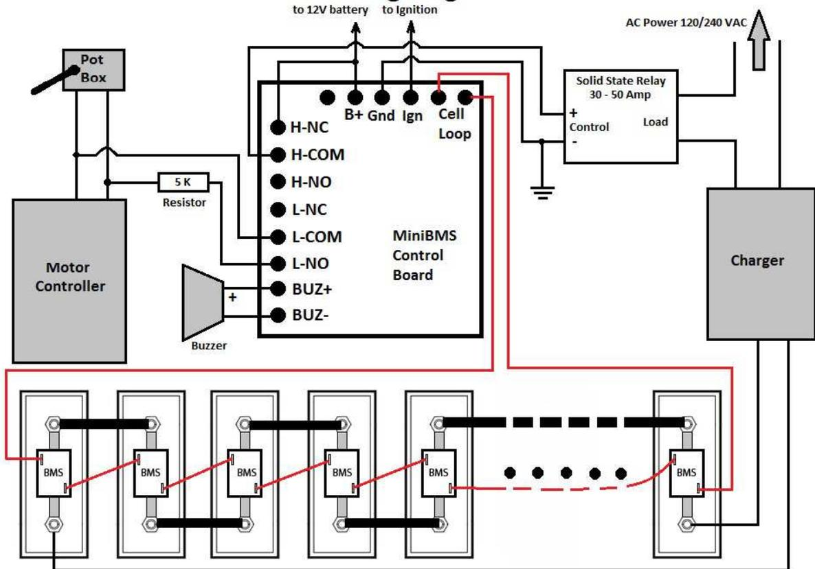
Next diagram shows only motor controller portion of MiniBMS wiring diagram for 3 wire resistive pot box and controller which expects 0-5V throttle input. Controllers which use this type of throttle input are Soliton1, Kelly, and others. Check controller's documentation for details. Do not use this diagram with Hall Effect throttles, please refer to the following diagram for Hall Effect throttles.
