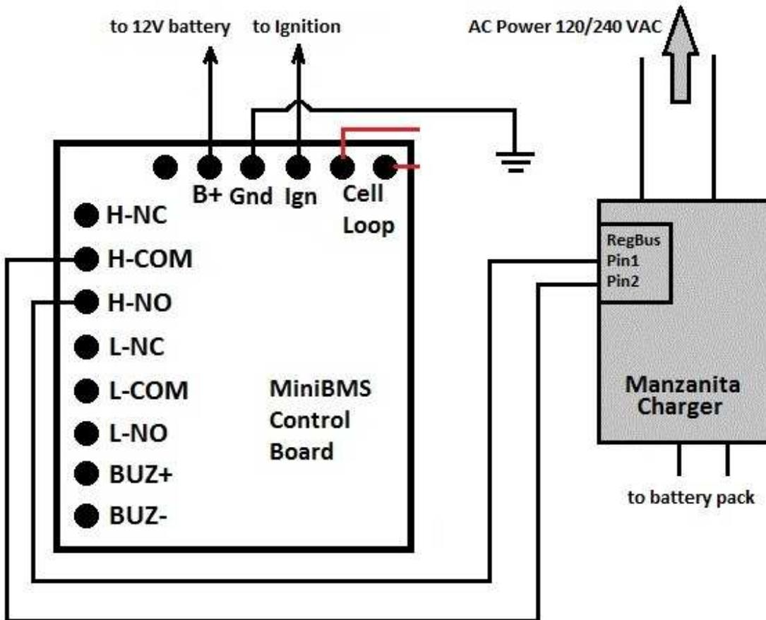
**NOTE: Manzanita chargers are not isolated, which can cause BMS damage if charger is mounted to vehicle chassis. You must mount the charger on non-conductive standoffs so charger body does not have electrical contact with vehicle chassis.**
