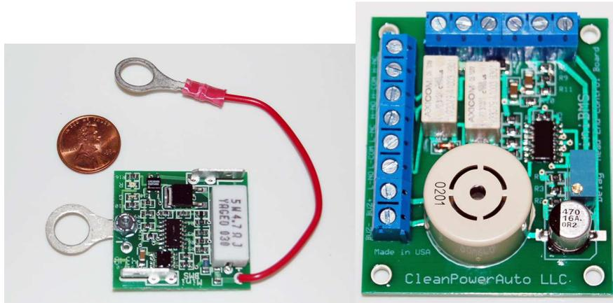
MiniBMS is a battery management system designed for LiFePo4 cells, used in Electric Vehicles. MiniBMS is designed to be a reliable and cost-effective solution; it has most basic functions, implemented via a simple analog circuit and one-wire interface, which also allows easy installation and troubleshooting.
