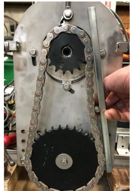
To adjust, tighten the tensioner nut. Test by pushing on the chain half way between the two sprockets until you notice firm resistance. The proper tension will yield about 3/8" motion away from a straight line, as shown in the picture. Tighten the motor mounting bolts to lock the motor in position.
