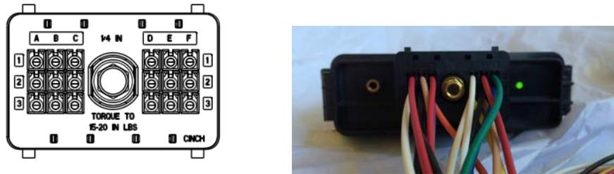
Figure 3 – EVCC Connector and Front Panel
