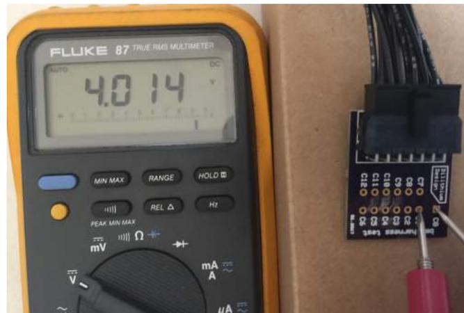
Figure 12 – Using the Cell Harness Tester
